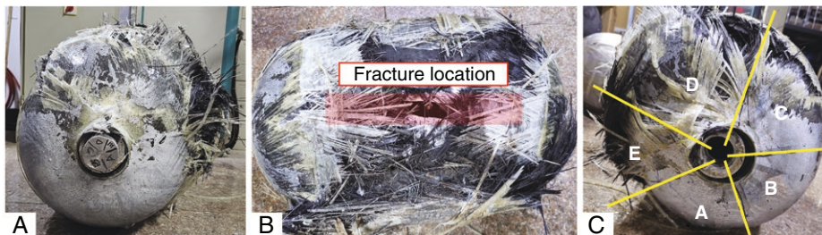
Figure 9. Three views of the COPV after the burst test: (a) left view; (b) front view; (c) right view.
